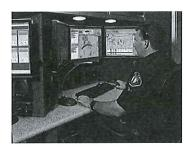
This illustration shows how the information collected from the wireless gas monitors appears on a visual display in a remote location. Both location and environmental conditions are displayed on the monitor. In this particular case, the information is being monitored in a HAZmat truck, which is commonly operated by the local municipal fire department.
